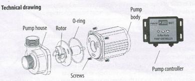
Unplug before cleaning. To clean the pump, remove the back cover, sealing cover and the impeller. Use a small brush or stream of water to remove any debris.
