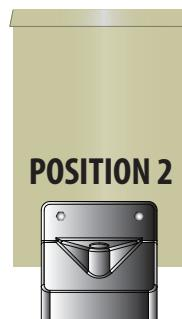
**Position 2 (Standard)** This level gives the weir its minimum length, suitable for higher pump speeds. The minimum length of the weir is to have a high water level under the screen to prevent a high speed pump from priming air.
