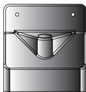
**Position 1** This level gives the weir its maximum length, suitable for lower pump speeds. The maximum length of the weir prevents the water level underneath the sieve from going too high for low speed pumps.
