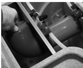
Figure 17.2 - Move 90° to by-pass
